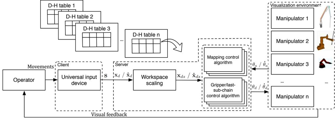
Fig. 1. The proposed control system architecture: a client-server architecture with the input device running as a client and communicating with a server where control algorithm logic is implemented.
