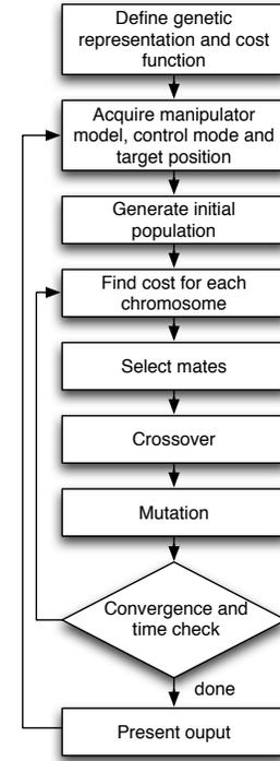
Fig. 3. Flow chart of the proposed mapping method.
