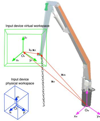
Fig. 2. The proposed architecture allows for expanding and shifting the small-scale physical workspace of the input device to a virtual expanded workspace, thus giving the robot arm the ability to make more accurate and precise movements.
