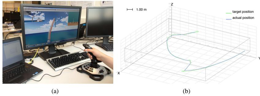
Fig. 4. The simulation of (a) the knuckle boom crane model and (b) the trajectory tracking of its Cartesian paths in X, Y and Z coordinates.
